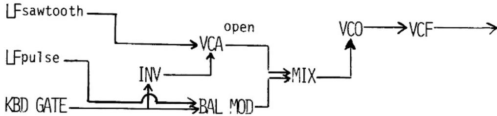
When the LF pulse is high, the VCO is controlled by the LF sawtooth. When the LF pulse is low, the VCO is controlled by the sine. In both cases the KBD voice always controls the VCO. As you can see, there are innumerable possibilities using the BM and the VCA in combination. Again, it's up to you to determine what is musically useful for your purposes.
