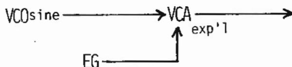
When you want a percussive attack but with a longer duration than is available with the exponentialized envelope, you can use this patch using the BM as an additional VCA.
