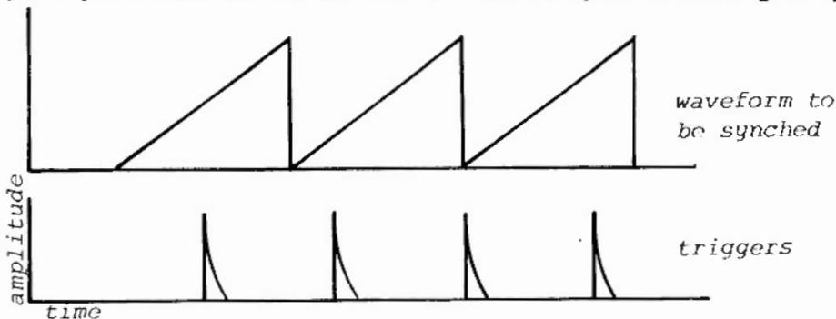
Instead of putting out a sawtooth, the slaved oscillator is outputting a waveform which looks like this.
