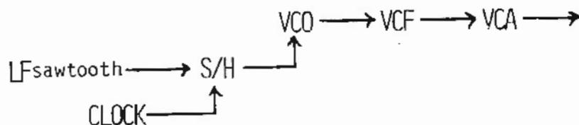
you can hear the result of the S/H. Make sure that the clock frequency is about 10 times greater than the frequency of the sawtooth. Also be sure that the S/H output level is turned up. This, by the way, is the only output attenuator on the entire synthesizer. All the others are input attenuators.
