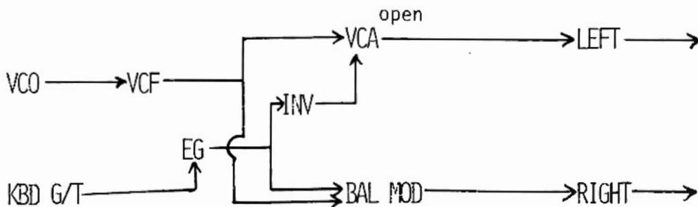
The EG voltage which opens the BM also gets inverted and closes the VCA. The result of the patch is that when a key is depressed, the sound comes from the right speaker, and it comes from the left speaker when there's no key depressed. Automatic panning is possible by using a LF pulse to fire the envelope generator.
