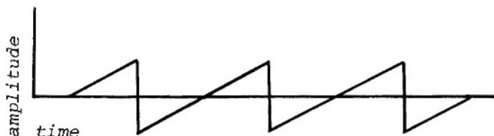
This waveform is balanced across 0 volts. It goes 5 volts positive and 5 volts negative. If you add a +5 DC bias to the signal, it would look like this.
