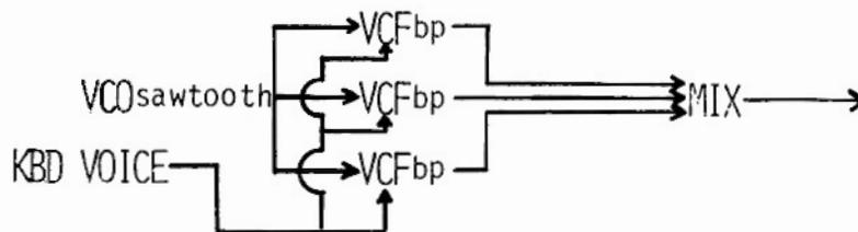
What you have patched is essentially a resonant, voltage controlled equalizer. It can produce timbres extremely close to those produced by acoustic instruments.
