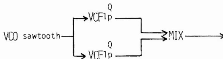
Another feature of the AR-327 is that it provides for voltage controllable resonance. Resonance, in any filter, is the result of a feedback loop in which the output signal is routed back into the input of the filter. It's possible, using your AR-314, to set up a voltage controlled resonance patch.
