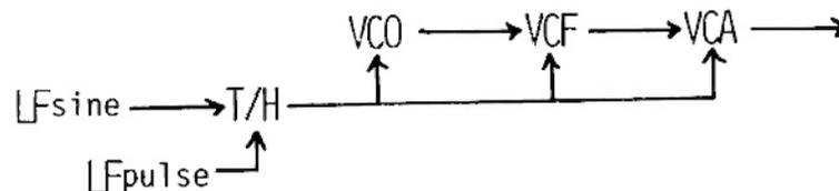
In order to patch the track and hold function, set the switch to "external" and patch any gate into the gate input. In block diagrams, it is represented as T/H and it is assumed that it requires a gate input. This patch has proven to have some useful applications as an "automatic percussion" patch.
