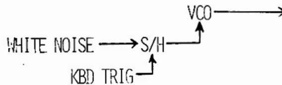
But any sharply rising voltage will do. When a gate or pulse is patched into the trigger input, the AR-318 will derive a trigger from the leading edge of the gate or pulse. This patch provides not only random pitches, but also random time events. Instant Subotnick!!
