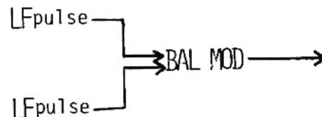
The BM is a four quadrant multiplier. This means that the BM will produce an output regardless of the polarity of either of the input signals. The formula for determining the output of the BM in the time domain is this.
