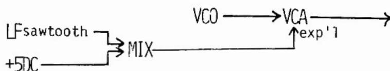
Try it first with the switch in the linear position, then switch it to the exponential mode. If you were to look at the sawtooth and the exponentialized sawtooth on a scope, you would see this happen to it.
