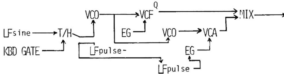
Another way of using either the S/H or the T/H is as a part of the audio path. Here's the patch.
