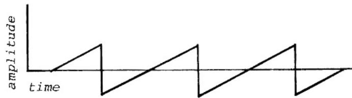
The amplitude is 10 volts peak to peak and it is a balanced waveform; the frequency is 100 Hz. (assuming you set it to 100Hz). Obviously the only difference between this waveform and a sine wave is its wave shape. Since the wave shape determines the motion of the speaker cone and the motion of the cone determines the timbre of the sound, the difference between the sound produced by a sine wave and a sawtooth wave is one of timbre.
