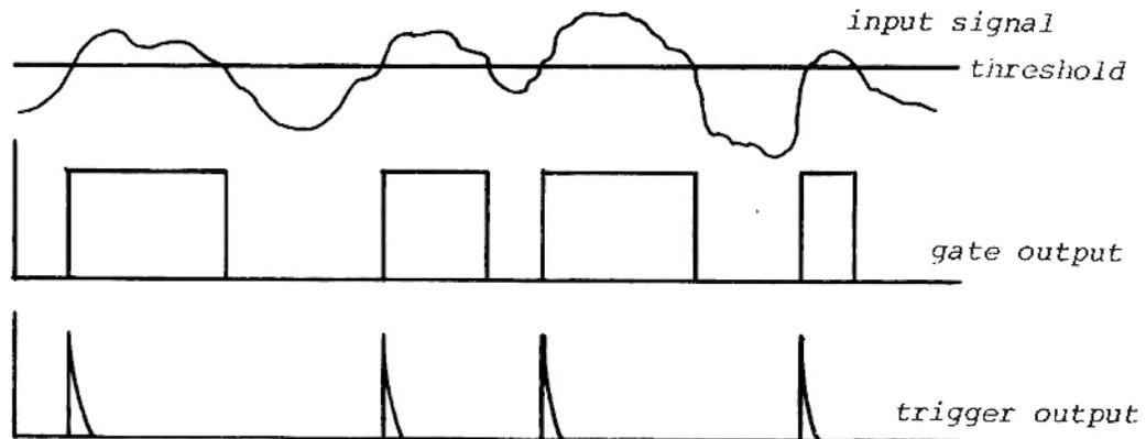
The comparator is useful in generating timing signals which are dependent upon another signal's amplitude. For example, in this patch whenever a loud note is played on the guitar, a gate is produced firing the envelope generator which opens the VCA allowing the series of random frequencies to pass.
