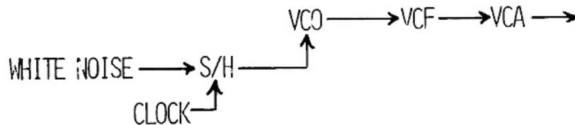
Try changing the output attenuator and limiting the overall pitch variance. The S/H output, like other voltages, can control frequency, amplitude, or wave shape. One way of controlling a signal's wave shape is shown in this patch which seems to have a lot of popular applications.
