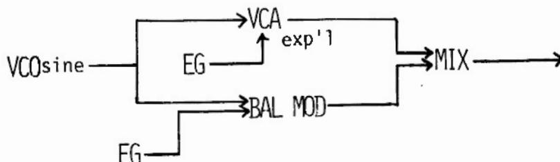
In block diagrams, the VCA mode switch is presumed to be in the linear position unless specifically marked "exp'l."
