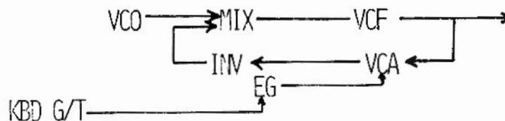
The inverter is in the patch to compensate for the phase shift caused by the filter at the cutoff frequency. The amplitude of the envelope determines how much of the output signal is fed back into the input and thus determines the amount of resonance. In the AR-327, this patch is made internally and any positive voltage patched into the resonance control inputs increases the amount of resonance.
