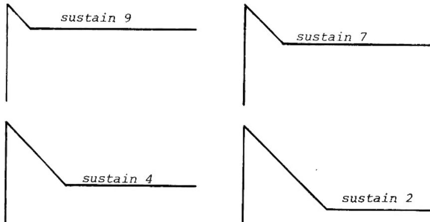
When the voltage has less distance to travel between the attack level and the sustain level, it gets there faster. In the previous patch where the sustain level was set to 10, the voltage had no distance to travel and so the decay time had no effect.
