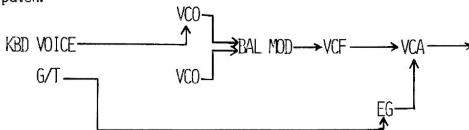
Set the envelope to simulate a bell's envelope (sharp attack, long decay, medium sustain, and long release) and try playing some different KBD notes. What happens in the BM is that the two sine waves are multiplied together and, in the frequency domain, this produces the amplitude modulation timbre that you hear. It's finally time to talk in some detail about modulation timbres.
