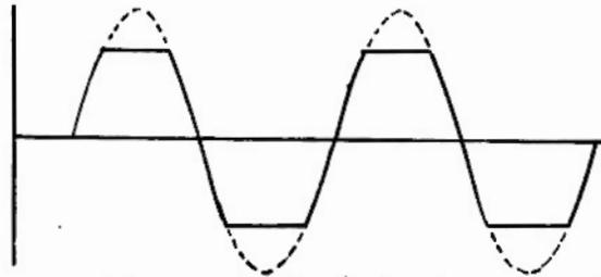
Clipping is a way of harmonically distorting a signal. It increases the energy in the harmonics. If you amplify the sine by the gain factor of 100, the pre-amp's output would begin to look like a square wave.
