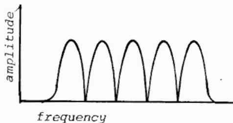
As you can see, there are 5 distinct peaks and 4 notches. Flipping the switch to the odd position, produces this comb filter slope which contains 4 peaks and 5 notches.
