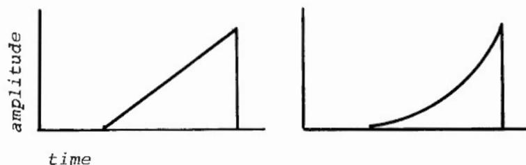
With the switch in the exponential mode, the VCA's output increases by 10 dB for each positive control volt. The result of exponentializing an envelope's voltage is to get a quicker and more percussive event. To synthesize most wooden percussion instruments, use an exponentialized envelope. Here's a wood block patch.
