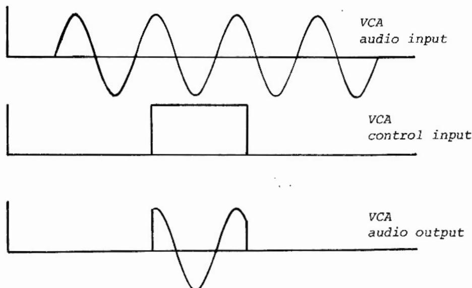
The pops you hear both at the beginning and the end of the gate are called "transients." They are caused by the gate's instantaneous voltage changes which snaps the speaker cone out, then back. Although transients help give acoustic instruments their characteristic sound, they are annoying in this patch. But then using the KBD gate is not the usual way of controlling a VCA. A more typical way is to use an
