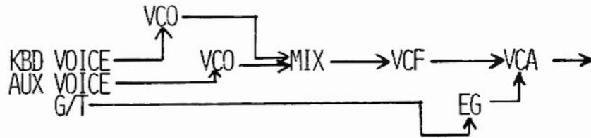
You can use the aux voice output to control other than an audio frequency VCO. In this patch, it controls the frequency of a LF pulse which fires an EG.
