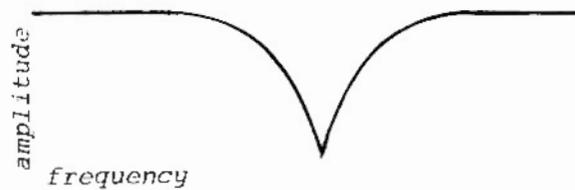
The resonance control, as you have probably surmised, will decrease the bandwidth of the notch and steepen the slope. The result is not as sonically obvious as with the peak and band pass filters because it is easier to hear one particular harmonic that has been accentuated than it is to hear one particular harmonic that has been attenuated. Still, the notch filter function is an important timbral modification device which offers some very subtle effects.
