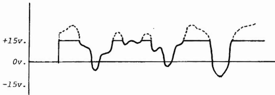
The way to avoid clipping, in this case, is to add a -10 DC bias. This again balances the resultant waveform across 0 volts. Keep in mind that when you are using a pulse wave as an audio signal that it is an unbalanced waveform and it might be necessary to use a negative DC with it to avoid clipping.
