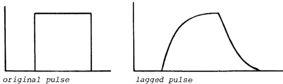
It rounds off all the sharply changing voltages. The lag time is variable from 1 mS. to 1 Sec. and is controllable by the lag (sec.) control. One of the ways in which it is commonly used is as an "envelope shaper." By lagging the KBD gate, you eliminate the transient pops from this patch.
