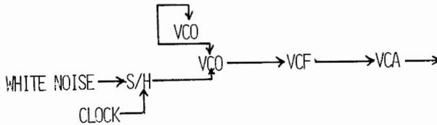
There are two additional ways of triggering the S/H. First, flip the switch to the external position, push the manual trigger button, and release it quickly. Each time you push the button, the S/H is provided with a trigger. It samples the signal and holds it until you push the button again. Another way is to patch any sharply rising voltage into the trigger input. Again the switch must be in the external position. One possible source of triggers is the keyboard trigger output.
