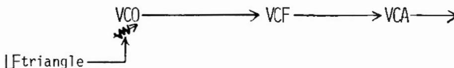
Before, we looked at a patch similar to this and, if you'll remember, the 10 volts LF sine drove the audio VCO up and down a total of 10 octaves. By attenuating the 10 volt sine down to maybe 1/20 or 1/30 volts, you can use it as a vibrato. Just so we can keep the terms straight, this pitch change is a vibrato while a similar amplitude change is a tremolo. A tremolo patch is this.
