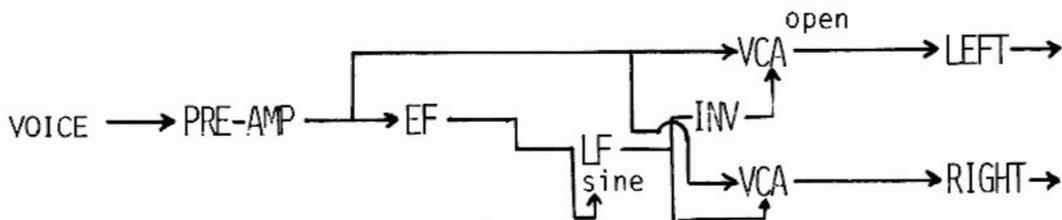
Using the pre-amp, the envelope follower, a VCA and an inverter, you can patch up a compressor.
