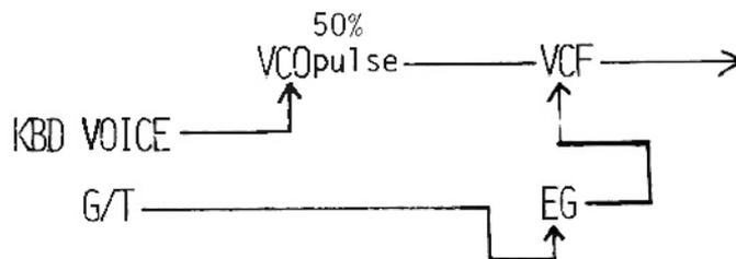
Set the filter  $F_c$  to minimum and make sure the resonance is set to minimum. Patch the envelope generator output into the filter control input #4 and patch the filter output into the output and power module. This patch does not use the VCA. There is a sonic difference between this patch and the previous patch. Listen to the sound as you play the keys and try to describe the difference.
