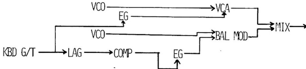
By using two percussive envelopes, you can create a single, stereo, "slap-back" echo. Be sure to hold the key down until both envelopes have fired.
