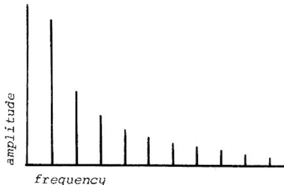
As you can see, a sawtooth wave contains harmonics that occur at all whole number (integer) multiples of the fundamental frequency and the relative amplitude of each harmonic is:
