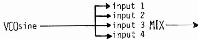
the output from the mixer is no longer a sine wave, but a clipped sine wave. Overload cannot harm your system and, in fact, you can intentionally clip signals to achieve harmonic distortion. Other than this, though the above patch has little use. A patch which you might often use, however, is this one.
