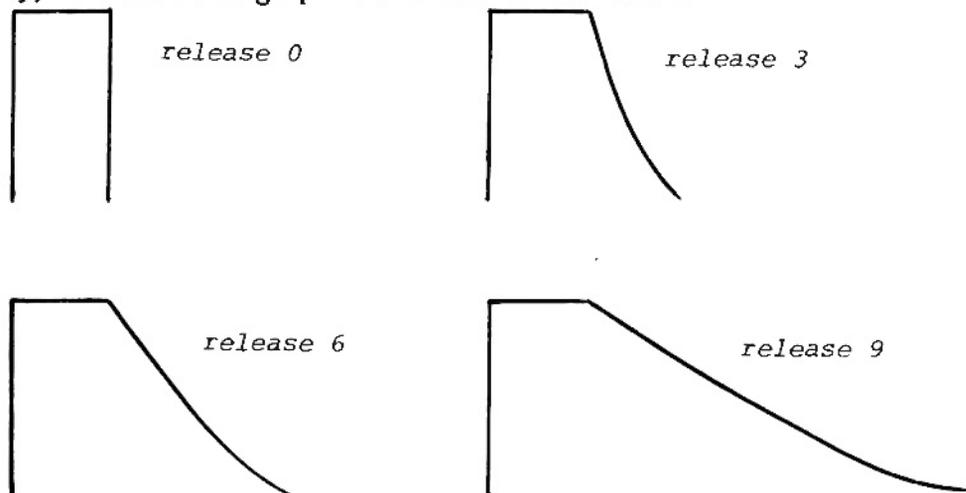
In the same way that changing the sustain level affects the decay time, changing it also affects the final release time. The release time determines how long the voltage takes to go from the sustain level to 0 volts. If the sustain level is low to begin with, it takes a shorter time to get to 0 volts.
