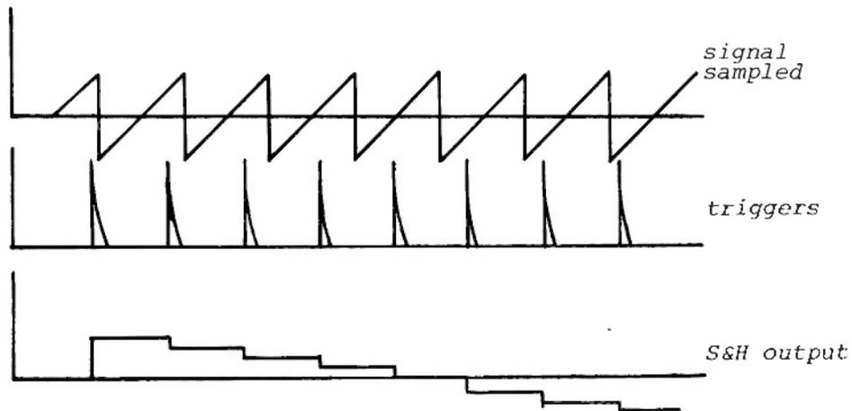
Of course, it's possible to sample any voltage. Sampling white noise in the following patch results in a series of random pitches.
