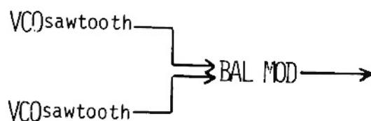
Each harmonic of each sawtooth must be added and subtracted from each harmonic of the other sawtooth. Even without doing all the arithmetic, you can see that the more harmonics that the waveforms have, the more complex the modulation timbre will be.
