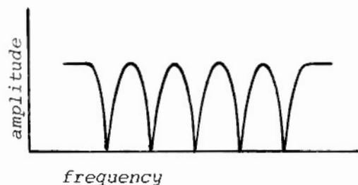
In almost all situations, the phaser produces a more "full" sound when the switch is in the even position rather than when it's in the odd position. Without getting into the math involved, here is what the switch does. At the input of the circuit, there is a phase splitting network. The outputs of the phase splitting network are coupled with the rest of the phase shifting circuit. The odd/even switch determines how they are coupled.
