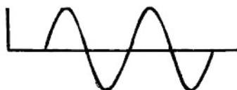
When the wave goes high, it forces the speaker cone out; when it goes low, it forces the cone back. Obviously, that sine wave causes the speaker cone to travel a greater distance than this sine.
