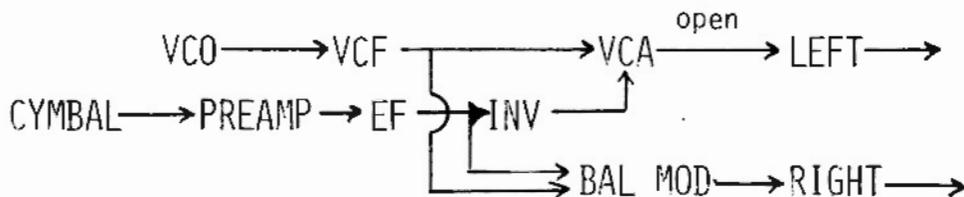
It is also possible to control the amplitude or the wave shape of the external signal itself. In this patch, a voice is the external signal and it is normally panning between two channels. The amplitude of the external signal determines the panning rate.
