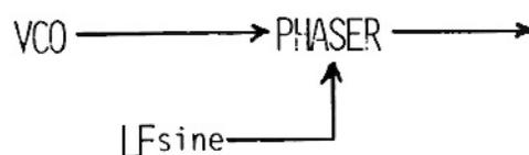
If you use the main output into one speaker and the aux output into another speaker and control the  $F_c$  with a slow sine wave or triangle, you can perceive apparent sonic motion between the two speakers.
