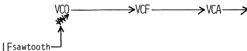
Just attenuate the 10 volt LF sawtooth down to one volt. Now un-plug the patch cord from the LF sawtooth and listen to the pitch of the VCO. When you plug the patch cord back in, you'll notice that the pitch glide starts lower than the original pitch. The problem is: how can you make the pitch start where you originally set it and then ascend upwards one octave? To accomplish this, you use the mixer.
