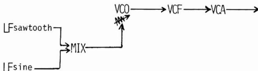
This patch offers a lot of possibilities. First you could try having the LF sawtooth at a very low frequency, say 0.2 Hz., and have the sine at about 7 Hz. Then you could attenuate the sine at the mixer so that it becomes a wide vibrato control. You should hear something that looks like this.
