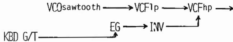
Second, it is possible to make a band pass or notch with different filter slopes on either side of the center frequency. That patch can be accomplished by having one of the filters resonant.
