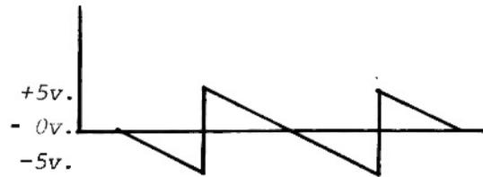
It remains a sawtooth and its harmonic spectrum remains the same. It is just put 180 degrees out of phase.
