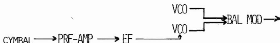
In this patch, the envelope follower's output is used to determine spacial location. The audio path appears first in the left channel then, when the cymbal is struck, jumps to the right channel and slowly pans back to the left channel as the cymbal decays.
