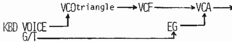
A triangle wave, like all other periodic waveforms, has a given harmonic structure. The harmonics of a triangle wave occur at all odd-numbered multiples of the fundamental frequency. If the fundamental (F) is equal to 400 Hz., then the harmonics occur at 1200 Hz., (3 x 400), at 2000 Hz., (5 x 400), at 2800 Hz., (7 x 400), at 3600 Hz., (9 x 400) and so forth. The amplitude of each harmonic is equal to:
