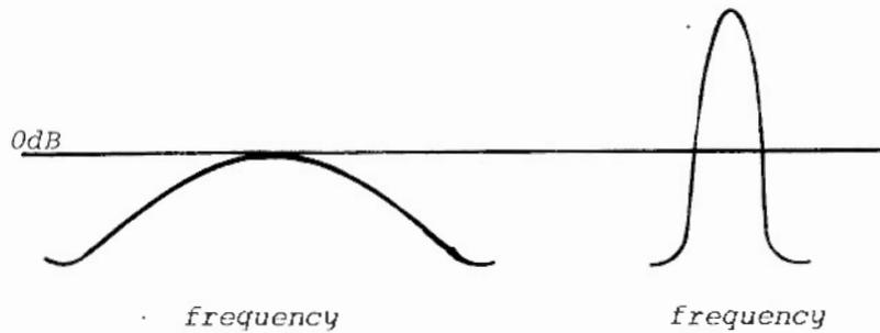
One band of a graphic equalizer is an example of a band pass filter. One way of using the band pass output is to make it resonant and tune it to one particular harmonic of the input signal. Controlling the frequency of the input signal and the Fc of the band pass filter with the same voltage assures that the same harmonic of the input signal will be resonated. Here's the patch.
