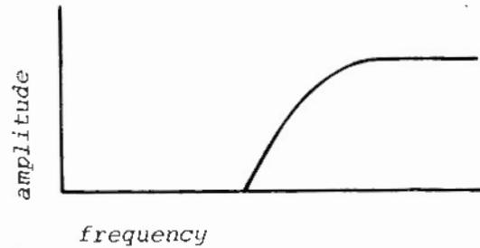
Any positive voltage applied to the filter's frequency control input will raise the cutoff frequency. When using the high pass filter function, it is usually necessary to invert the control voltage. Some interesting timbral changes are possible with this simple patch.
