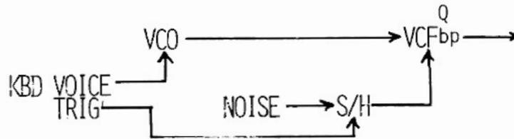
The band pass function of the AR-327 can be used in conjunction with other AR-327's patched either in series or in parallel. In series, the slopes of the filter functions are added together producing an extremely narrow bandwidth. Making them resonant, of course, further decreases the band width. The Fc's should be tuned together.
