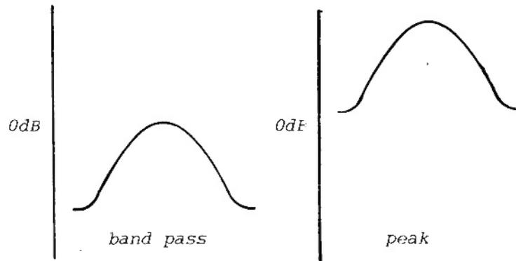
As an experiment, patch a sawtooth wave of some low audio frequency into the AR-327 and listen to the peak output. Tune the  $F_c$  so that it is equal to the fundamental of the sawtooth and use the maximum amount of resonance. Slowly increase the  $F_c$  and count the number of the individual harmonics that you can identify. You should be able to hear at least 32 individual harmonics.
