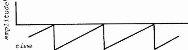
The sawtooth wave generated by the dual LFO module is already an unbalanced, positive sawtooth
