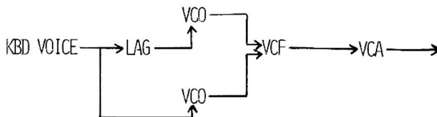
This patch is particularly useful in simulating the chorus effect of instruments playing in unison. In this application, use just the smallest amount of lag time.
