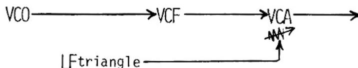
In an acoustic instrument, it is very difficult to produce either just a vibrato or just a tremolo; they almost always occur simultaneously. Naturally any other LF waveform can be substituted for the triangle. A pulse or square wave is particularly useful in synthesizing fast trills. If the controlling VCO is in the audio range, the result will again be a frequency modulation timbre. We'll again defer discussing this in detail until later. For now, here's another problem.
