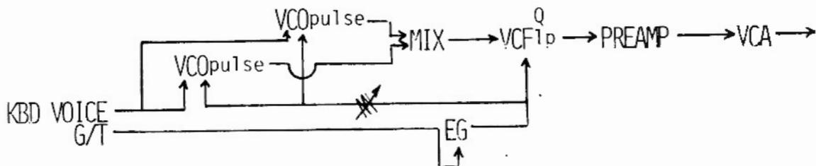
Although the output of the pre-amp is normalled into the envelope follower's input, inserting a patch cord into the pre-amp's output does not break this connection. This connection is only broken by inserting a patch cord into the envelope follower's input.
