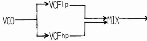
Set the  $F_c$  of your low pass filter to about 300 Hz. This will, of course, pass frequencies below 300 Hz. and attenuate frequencies above 300 Hz. Next, set the  $F_c$  on the high pass filter function to about 800 Hz., passing the frequencies above that point. When the same signal is patched into these two filters in parallel and the outputs of the two filters mixed together, it is as if you have superimposed the two filter slopes. Here is the result.
