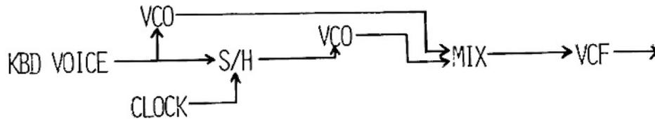
First, hold the lowest note on the KBD down and tune the 2 VCO's to unison. Second, play an octave higher on the KBD and, by using the output attenuator on the sample and hold, again tune the VCO's to unison. Third, set the clock frequency to about 1 Hz. Now, by playing a different note on the KBD each time the clock is halfway through its cycle, you can get one oscillator to follow the other one always ending up at unison.
