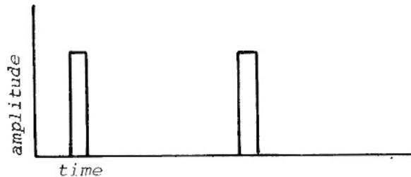
Another term used, in addition to pulse width, to describe pulse waves is "duty cycle." This term is just the fractional equivalent of the pulse wave percentage. In the case of a 50% pulse (also called a square wave) the duty cycle is  $1/2$ . This fraction means that for every cycle of the pulse wave, the voltage spends one half of its time high. The time domain graph of a square wave, or 50% pulse, is this;
