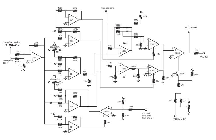
NOTES: all OP-AMPS powered by +/- 14.5 volts except TL082 powered by +18(++)/-14.5 waveshape sweeps continuously from triangle to saw to square to pulse you may want to eliminate the level VCA and replace the 3080 with a regular OP-AMP I take no responsibility for parts being the wrong values as the original schematic was illegible all pots were unlabeled but I think 100k linear will work
