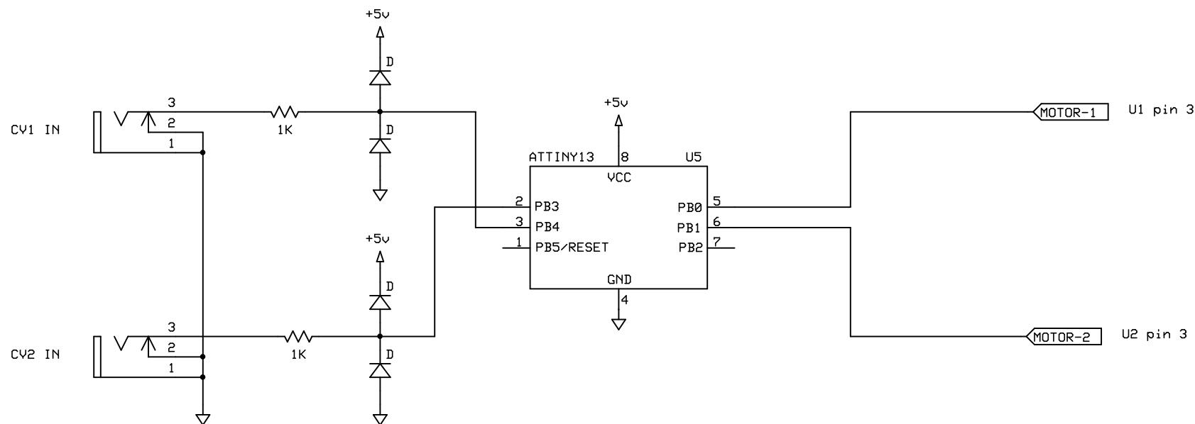
36.5 Hz MOTOR CONTROL FOR RAMSEY ELECTRONICS LLS1 MODULE
